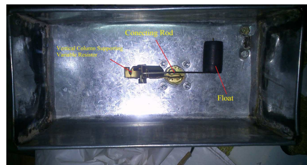
Fig2: Float arrangement system as a sensor.
